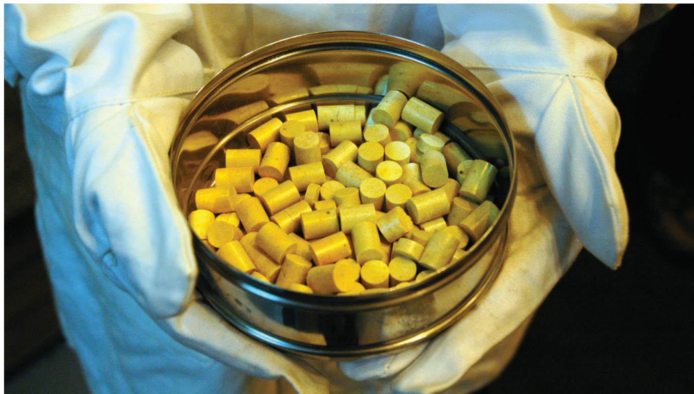
Thorium dioxide pellets could be the nuclear fuel of the future if proliferation concerns can be addressed.
